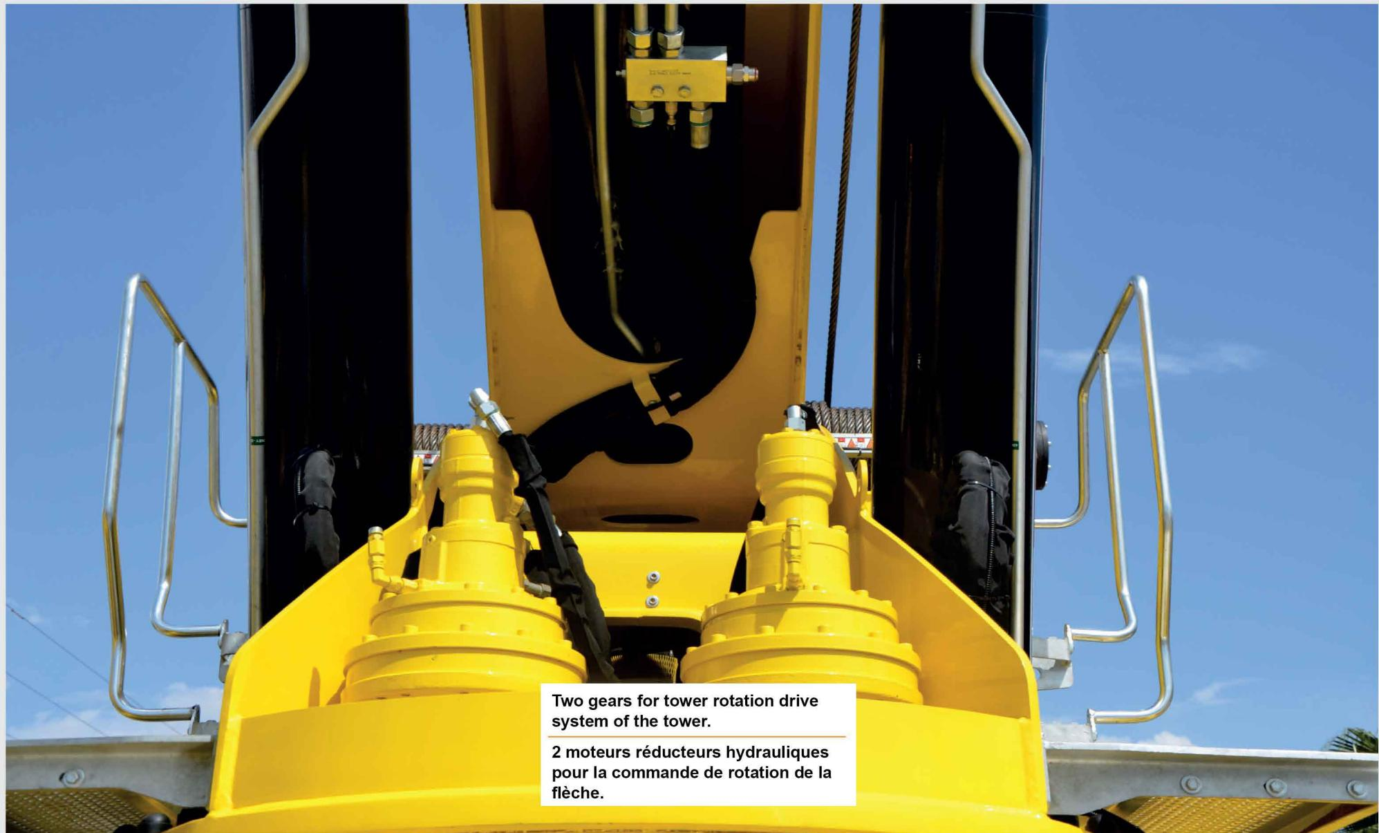
Two gears for tower rotation drive system of the tower.
